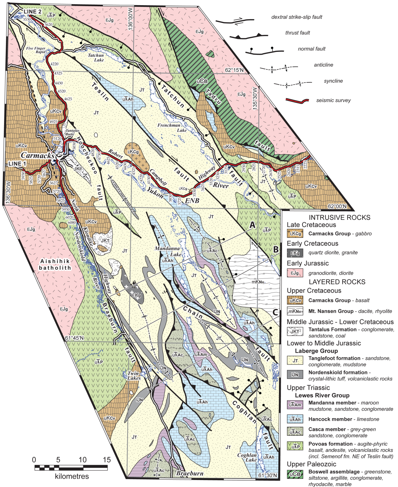
Figure 4. Geological map of the northern Whitehorse trough (after Colpron et al., 2007) showing the locations of the two seismic lines. In the vicinity of Carmacks, seismic lines 1 and 2 are co-located from just north of Carmacks to the junction with the Robert Campbell Highway. Seismic station numbers are not shown for this segment to avoid clutter. Upper Triassic volcanic and volcanoclastic rocks northeast of Teslin fault are part of the Semenof formation (Quesnellia). For simplicity they are grouped here (and in seismic sections) with the correlative Povoas formation (Stikinia). Based on regional considerations, the Teslin fault is interpreted to have a compound history of thrust and strike-slip faulting (see text). Sections A, B and C are depicted in Figure 5. ENB – Eagle’s Nest Bluff.
